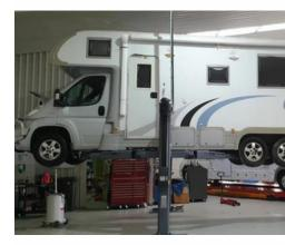
The AUTOPSTENHOJ Maestro 2.65F TT/TT 6.5 tonne two post lift features newly designed 4 stage telescopic arms, with a standard minimum height of only 98mm.
